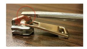
3) BY Pressing On The Top, Cap Goes Into The Slider
